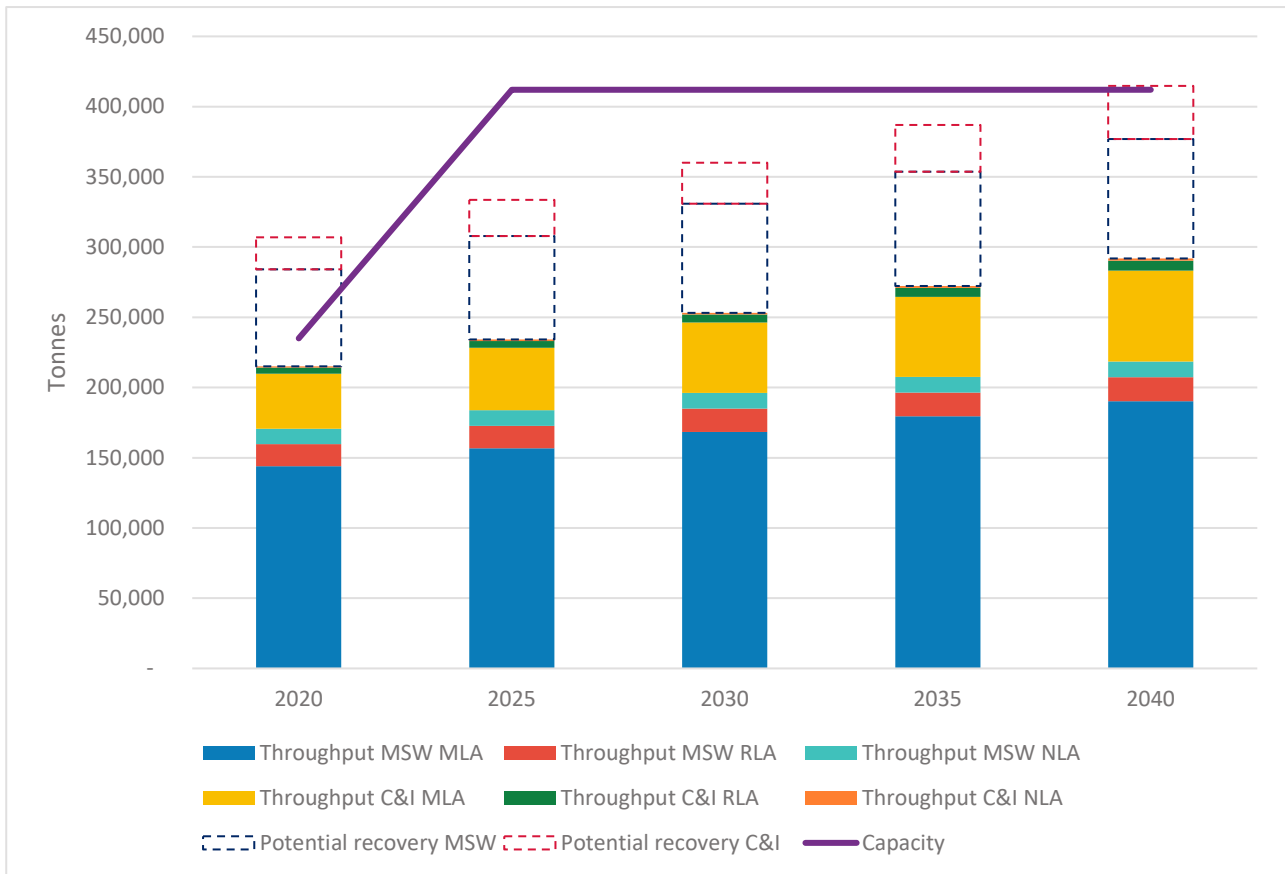
Figure 4. Estimated NSW glass processing throughput and potential additional recovery (through improved capture from residual waste) versus business as usual processing capacity iv
